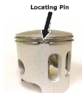
Figure 2 - Ring Locating Pin
